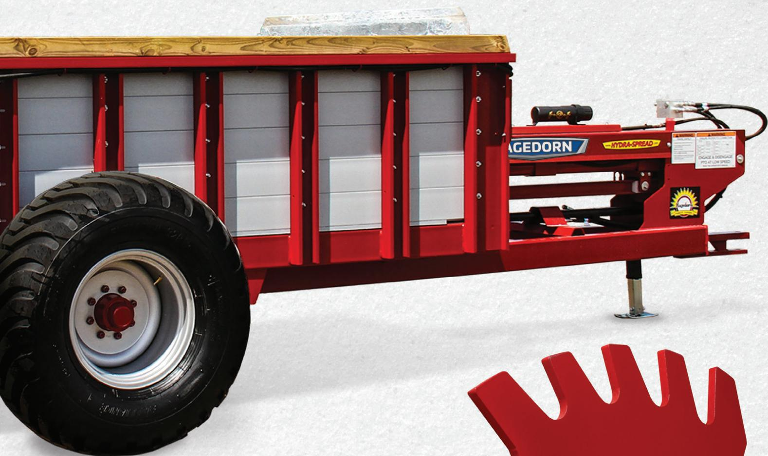
RipGrip beater paddles are designed with a unique shape to aggressively rip the manure and hold onto it for a fraction of a second, resulting in a spread pattern that puts manure behind the spreader rather than into the air. Position and spacing of the paddle give the widest and most uniform spread pattern available in horizontal spreaders.
