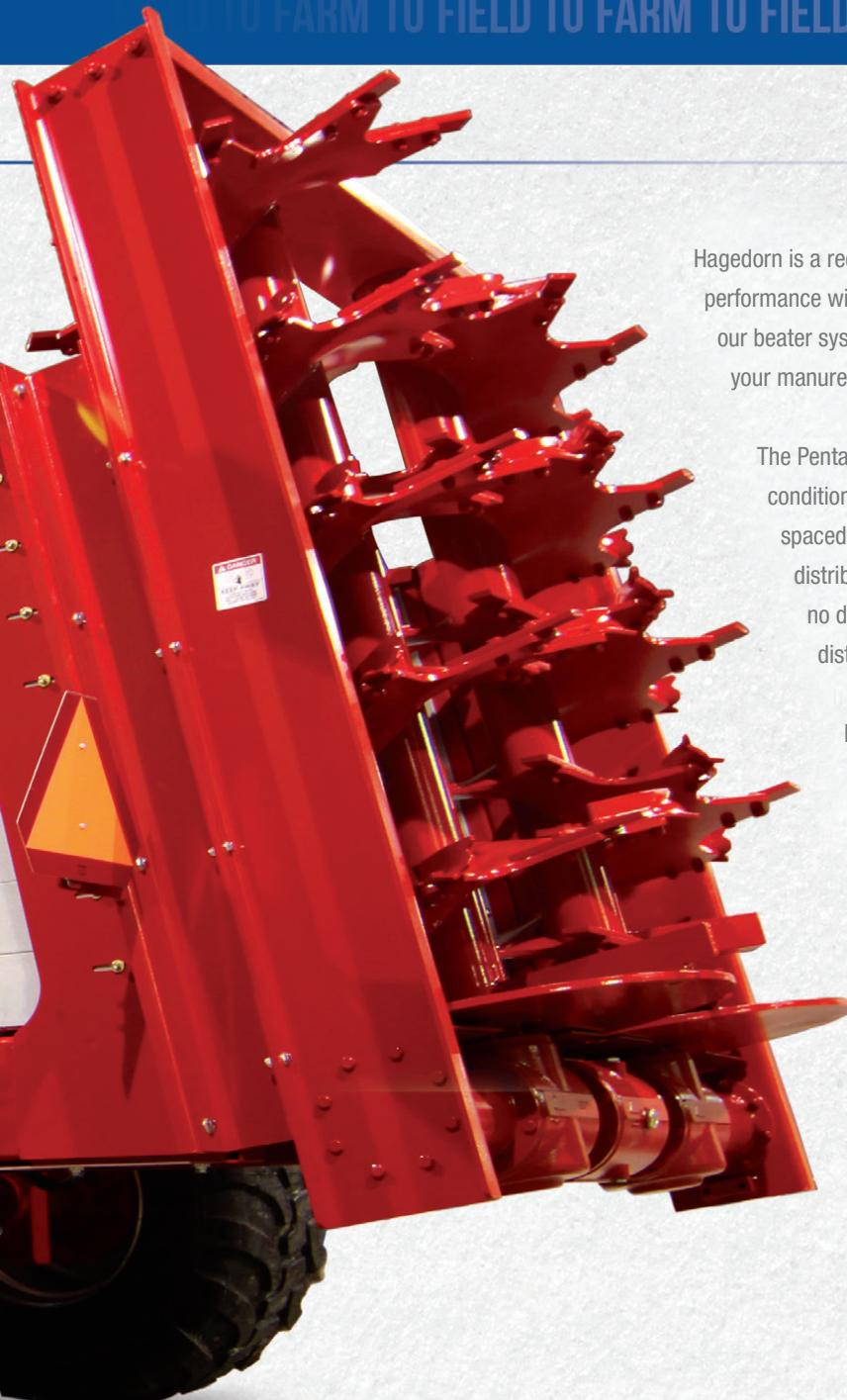
Hagedorn is a recognized leader in hydraulic push-off technology. Increased spreading performance with our Penta vertical beaters, combined with innovative design, means that our beater system delivers performance and control that maximize the nutrient value of your manure.
