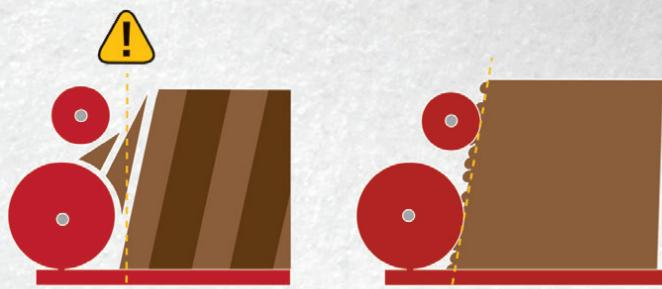
The RipGrip beaters are optimal for fine, wide and uniform horizontal spreading. The RipGrip system, which includes a stepped beater position and aggressive beater paddles, allows for improved manure processing.
